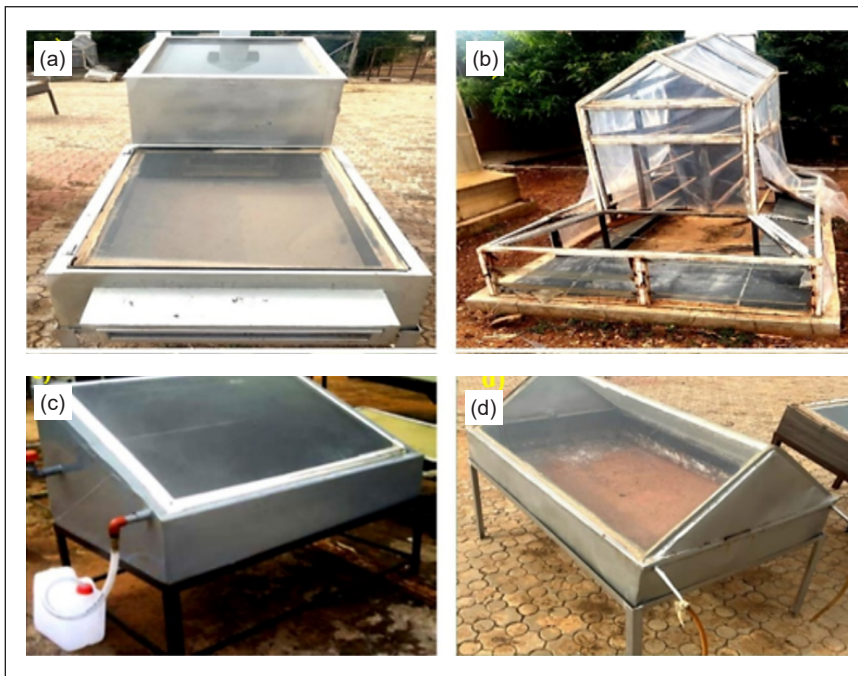
Figure 1. (a) Corroded absorber in a solar dryer; (b) Corroded solar dryer; (c) Corroded absorber in a solar still; and (d) Corroded absorber solar still. Pictures taken from Sokoto Energy Research Centre, Usmanu Danfodiyo University, Sokoto, Nigeria
