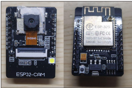
Figure 2. Front and rear view of ESP32 CAM
