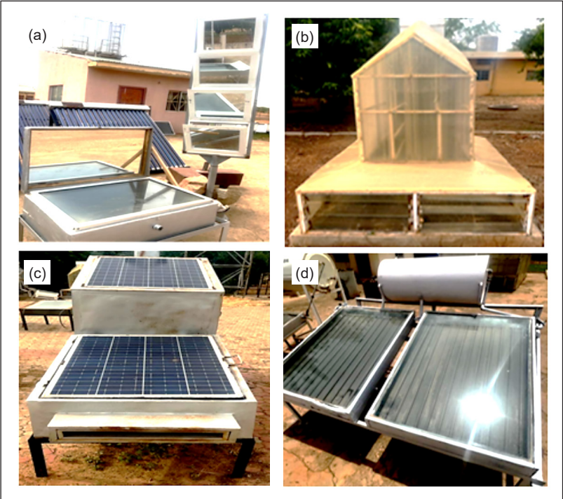
Figure 3. Concentrating and non-concentrating STSs (a) Concentrating solar still; (b) non-concentrating solar dryer; (c) hybrid solar dryer, and (d) non-concentrating evacuated solar water heater. Pictures taken from Sokoto Energy Research Centre, Usmanu Danfodiyo University, Sokoto, Nigeria
